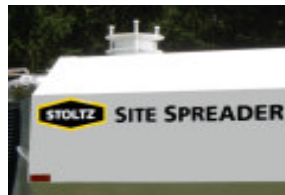
9" Pressure Relief set at 2psi - Standard.
