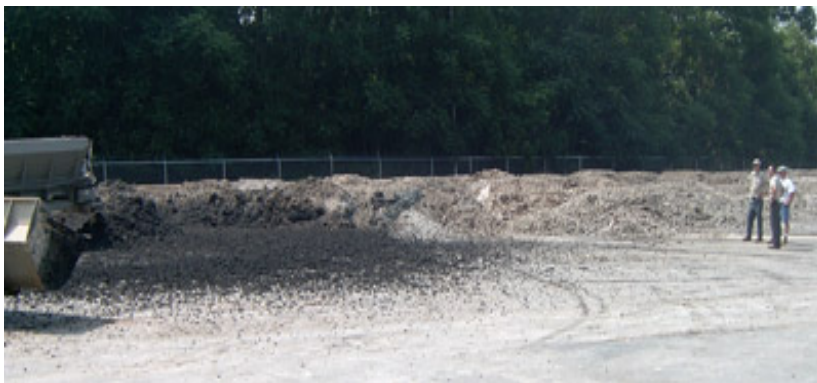
Spread pattern testing with wastewater treatment sludge.
