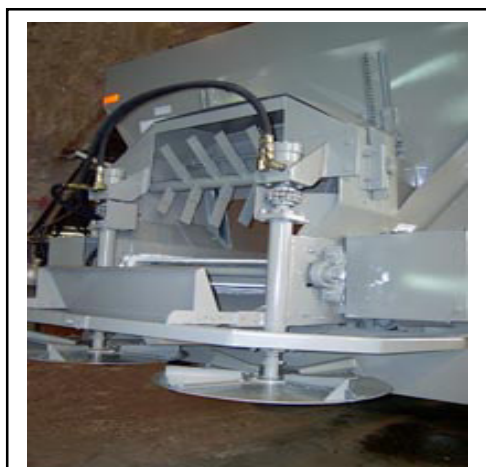
Low rpm “shredder” breaks up lumps for a smooth flow of material onto the spinners.
