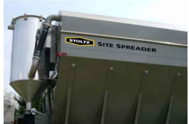
Filter can removes dust from vent air during filling.
